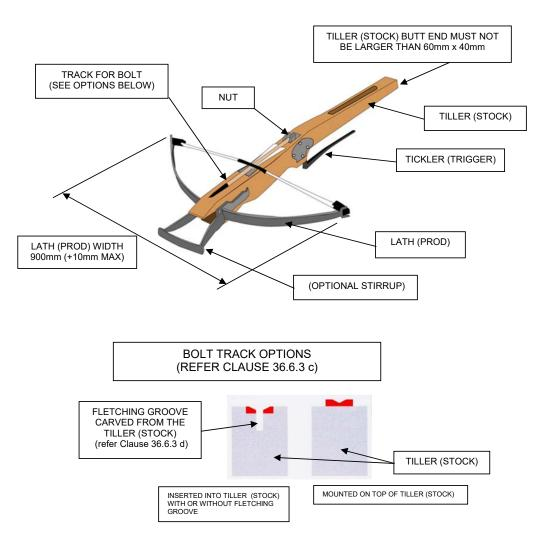
APPENDIX 4 - DIAGRAM OF MEDIEVAL CROSSBOW TICKLER (TRIGGER) MECHANISM
